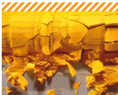
Uranium concentrate (yellowcake), resulting from ore processing. It is then transported for subsequent enrichment operations.
