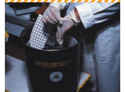
Example of LLW/ILW-SL (low level and intermediate level, short-lived waste) from laboratory operations.
