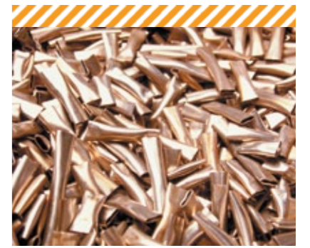
Example of ILW-LL (intermediate level, long-lived) waste – Fuel end-pieces.
