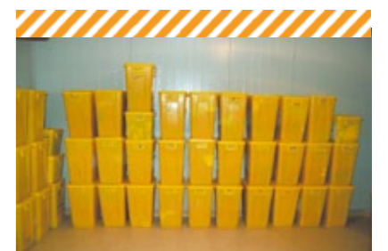
Tanks containing daily waste from iodine 131 treatment, stored in a refrigerated room during decay, nuclear medicine department, Brabois hospital for adults, Nancy university hospital.
