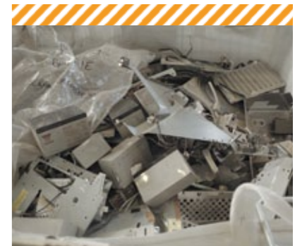
Example of VLL (very low level) waste: pieces of metal and plastic from the decommissioning of nuclear facilities.
