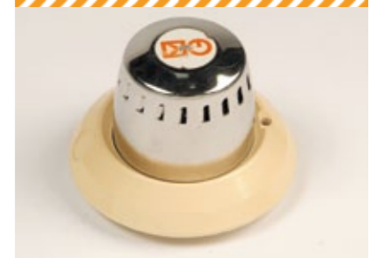
Some objects of our everyday lives can contain radioactivity. They are usually LLW-LL (low level, long-lived) waste. For example, certain ionisation chamber smoke detectors contain Americium 241 which is radioactive.
