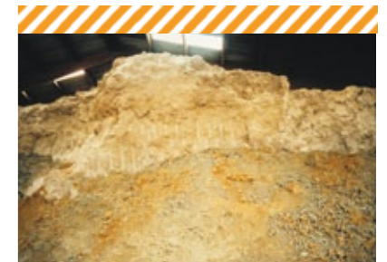
Residues from the rare earths extraction process (Solvay). This waste is referred to as TENORM.
